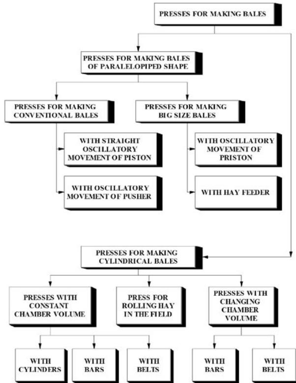
Figure 1. Scheme of classification of presses for hay
