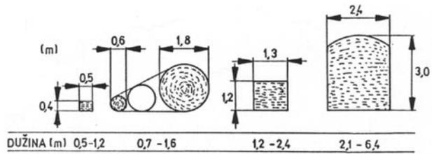
Figure 2. Geometric parameters of bales
