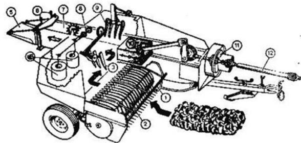
Figure 3 : Scheme of a hay press (1- shield, 2- collector, 3- pusher, 4-linking means, 5-output channel, 6-device for setting level of compression for bales, 7- chamber, 8-device for binding bales, 9 – compressing device, 10 – piston, 11- fly wheel, 12- cardan shaft)
