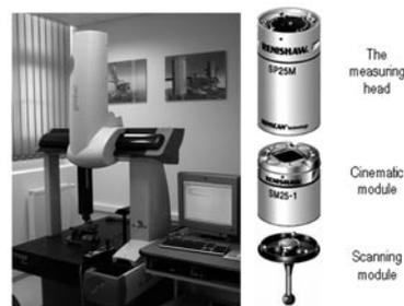
Fig. 6. DEA Image Clima 7.7.5 CMM (left) and probing head SP25M (right)
