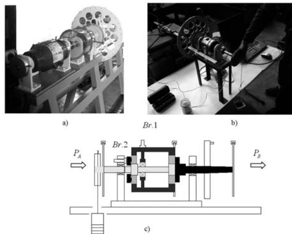
Fig. 3. Bench for testing planetary gear trains
