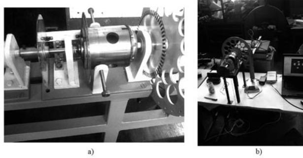
Fig. 4. Bench for testing planetary gear trains - fragments
