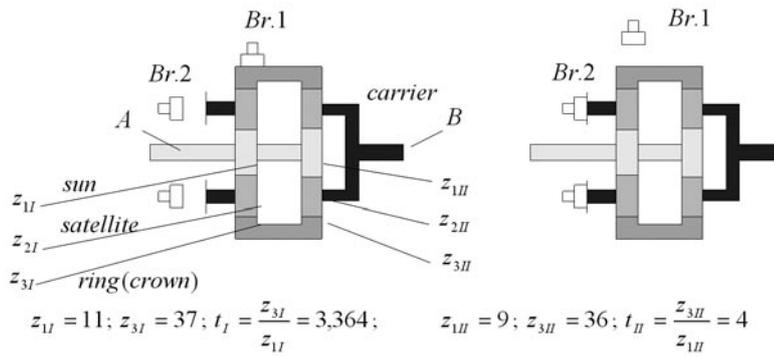
Fig.1 Experimental gear train
