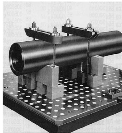
Fig. 3 Fixing of the component on the base plate with the openings
