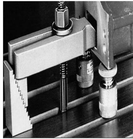
Fig. 2 Fixing by the screw and the nut for T-slot
