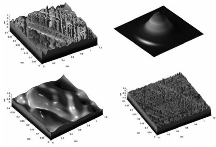
Fig. 5. Gaussian digital filtration – example with surface after honning
