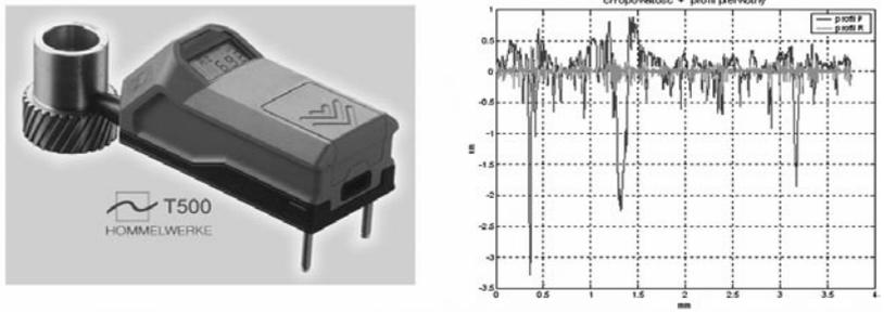
Fig. 4. Portable profilometer HOMMELWERKE T50, and the measured profile unfiltered and filtered
