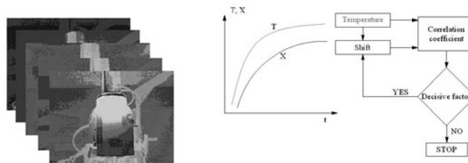
Fig. 7. Algorithm aiding the choice of thermal sensor locations giving the best correlation between recorded increases of temperature and unintended shifts (thermal deformation) [14]
