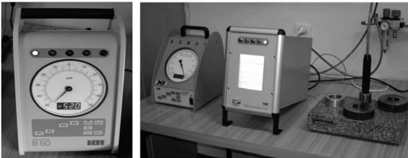
Fig. 3. PNEUTRONIK devices type B50 (left), B25 (middle) and C2K (right) with master rings
