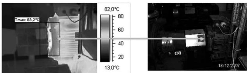
Fig. 6. Thermal imaging of the electric motor with damaged bearing
