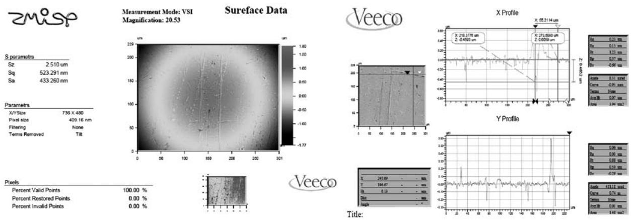
Fig. 5. Surface of the calibrating sphere (left) and its filtered profiles (right)
