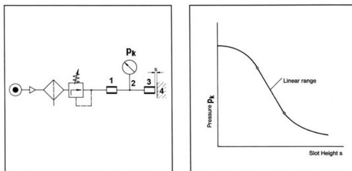
Fig. 2. Typical high-pressure open jet type air gauge (left) and his static characteristics (right) (based on [6])
