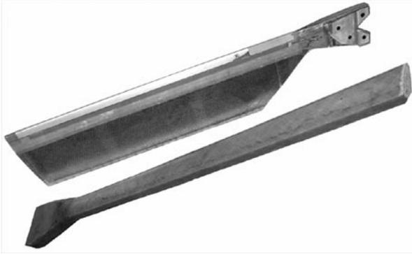
Fig. 1. Tail rotor blade and composite spar
