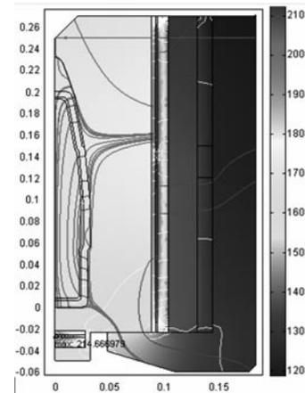
Fig. 6. Plot of the simulated stationary temperature field in a mould cross section
