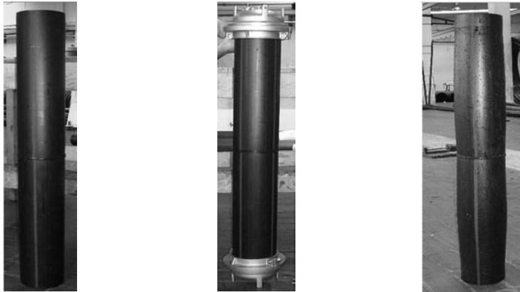
Fig.5. the samples before and after the examinations on impermeability
