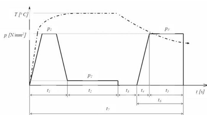
Fig.2. Regime of heated tool plate shaped butt welding
