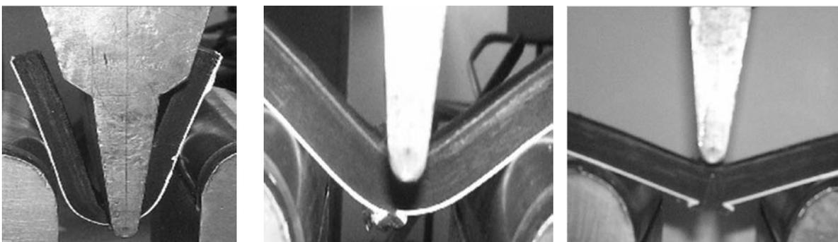
Fig.4. Samples examined by bending
