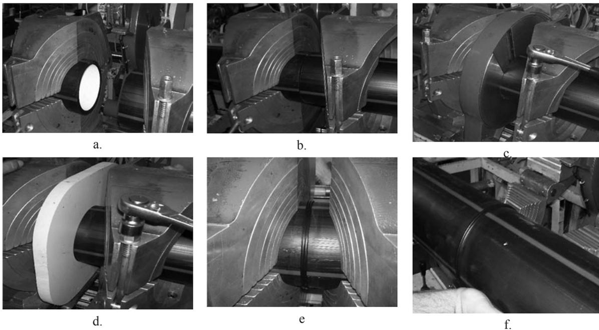
Fig.1. Phases of heated tool plate shaped butt welding
